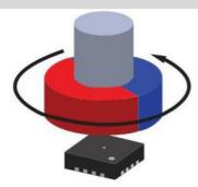
FA21 uses the classic tail wing to measure the direction of the wind, and the three-cup rotation measures the wind speed. The electromechanical conversion circuit is realized by the combination of the magnet on the end of the measuring shaft and the imported magnetic encoding chip on the circuit board. , Can ensure that the wind speed and direction signal output by the sensor is accurate and reliable.
