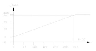
4-20mA Pulse output characteristic curve:
